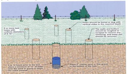
The perc test cannot be run when the air temperature is below 40° F or if the soil is frozen or snow covered.
